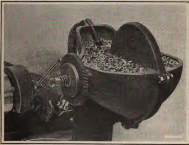
Fig. 17. Hopper from which Blank Nuts are fed automatically
